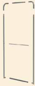
Add the central reinforcement bars and connect all the tubes using the easy matching system
